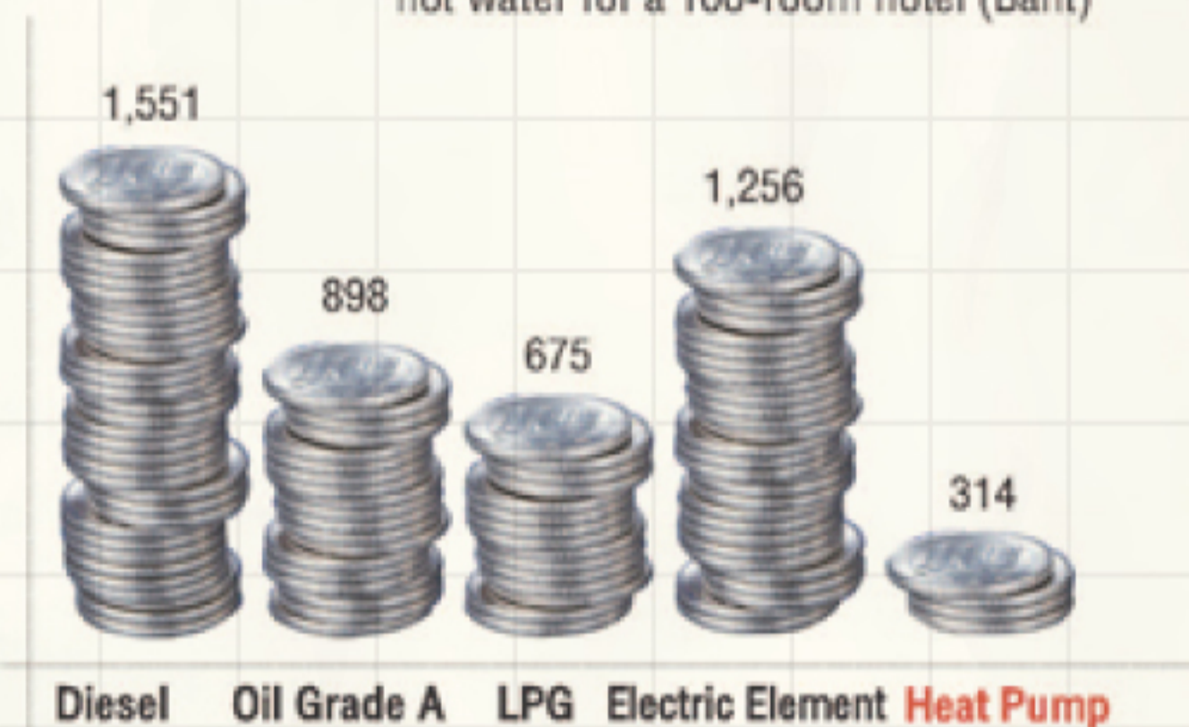
■ Comparison with the daily cost of heating hot water for a 100-room hotel (Baht)
